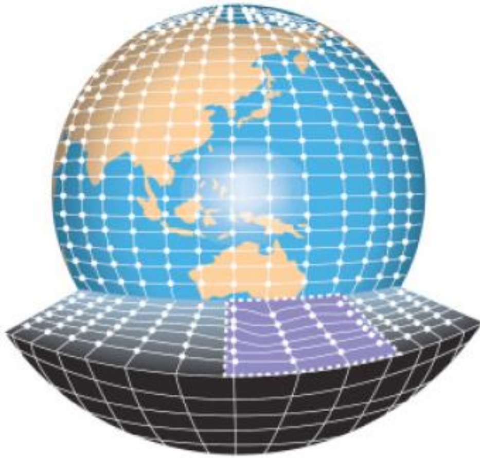
Figure 1. A schematic showing grid points, both horizontal and vertical, at which calculations are made in a numerical prediction model of the atmosphere. (Source: Bureau of Meteorology)
