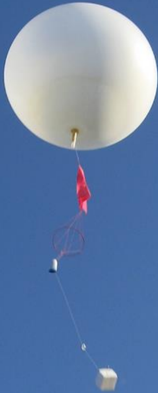
Balloon with parachute and radiosonde
