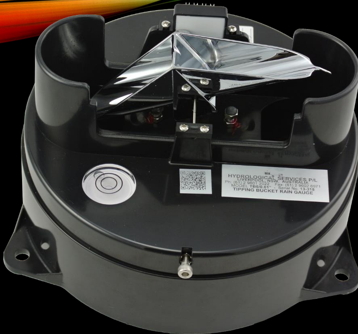
The internal mechanism of a tipping bucket rain-gauge
